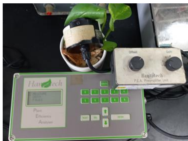
Fig. 1. Measurement of chlorophyll fluorescence of Epipremnum aureum by Chlorophyll Fluorometer.
