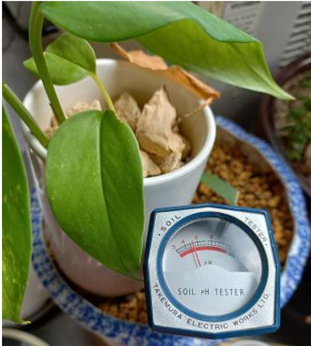
Fig. 2. Measurement of soil pH by portable pH meter of Epipremnum aureum growing in the pot.
